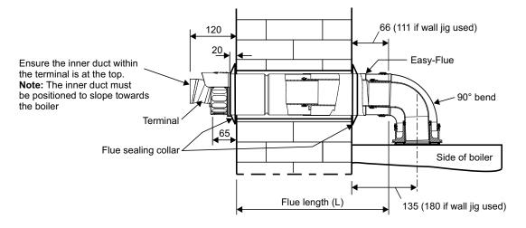
Fig. 5.11 - Push fit rear flue
