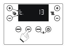
To select the desired parameter (e.g. t.13) press the 'INFO' button to scroll through the parameters within the family (e.g. t.) previously selected and then confirm by pressing the 'MODE' button.
