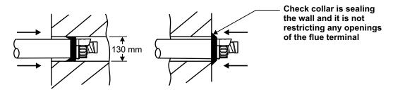
Fig. 5.10b - Fitting the flue from inside
