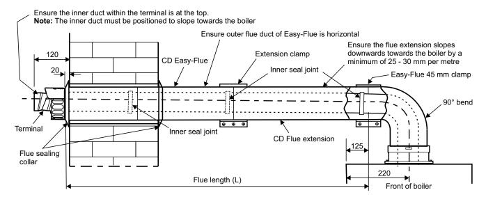
Fig. 5.13b - Clamped side flue
