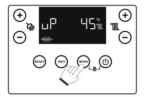
After confirming the lower set point, the upper temperature set point is displayed (default 45°C, range 25 - 50°C), which can be edited in the same way. Confirmation by pressing the 'MODE' button will save the value and the Screed Heater function is activated.
