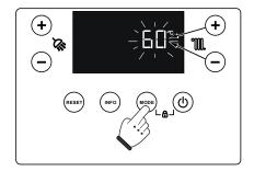
If the parameter can be adjusted, it activates the option to adjust the parameter using the CH (  $^{\mathbf{M}}$  ) +/- buttons.
