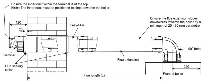
Fig. 5.13 - Push fit side flue
