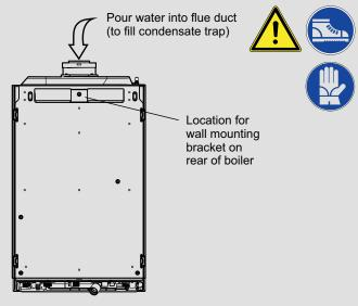
Fig. 5.3 - rear of boiler
