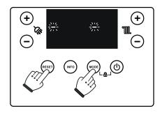
To access the programming phase, press and hold the 'MODE' and 'RESET' buttons at the same time for more than 5 seconds, the display will show two dashes (-) single blinks and you must enter the password '69' to access the programming menus.
