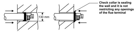
Fig. 5.10 - Fitting the flue from inside
