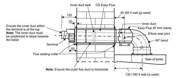
Fig. 5.11b - Clamped rear flue
