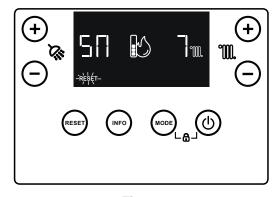
The screen will now alternately display the countdown of days (short duration) and current flow temperature (long duration) simultaneously with the normal operating information (CH request, flame, fault symbols etc.).
