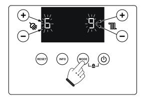
To enter the digit on the left, use the DHW (  $\mbox{\ensuremath{\mbox{$\%$}}}$ ) +/- buttons. To enter the digit on the right use the CH (  $\mbox{\ensuremath{\mbox{$\%$}}}$ L) +/- buttons. Press the '**MODE**' button to confirm the password.
