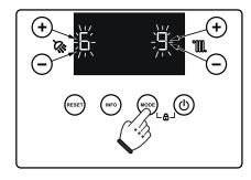
To enter the first digit of the password use the DHW (  $\mbox{$\mbox{$$\%$}$}$  ) +/- buttons, to enter the second digit use the CH (  $\mbox{$\mbox{$10$}$}$ L) +/- buttons.
