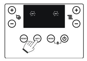
Press and hold the '**INFO**' button for more than 5 seconds. The display will show two dashes ' - - ' flashing. Now enter the password "6 9" to access the programming menus.
