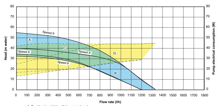
A+B = Head available with by-pass closed B = Head available with by-pass open
