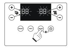
The parameter adjustment is saved by pressing the 'MODE' button after its value has been adjusted, displayed by '⊞⊞ ⊞⊞' flashing for 2 seconds.
