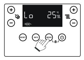
Activation of the function will display the lower temperature set (default 25°C, range 20 - 45°C), which can be edited by pressing the 'MODE' button and using the CH ( ML) +/- buttons and finally confirmed by always pressing the 'MODE' button. The adjusted set flashes for 2 seconds after the last time a button was pressed.
